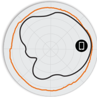
Figure 3. T610o 5GHz Azimuth Antenna Patterns
