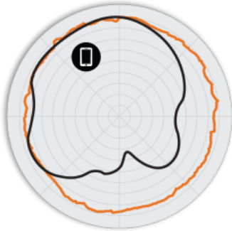
Figure 2. T610o 2.4GHz Azimuth Antenna Patterns
